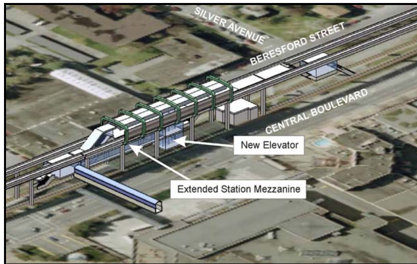
Figure 9 Extended Station Mezzanine
